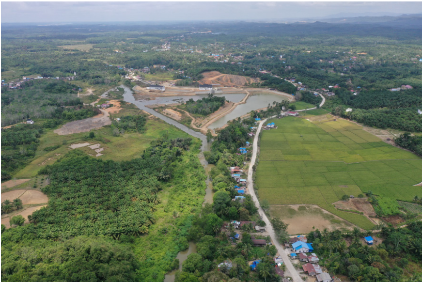
Figure 57. Sepaku Intake and the diverted Sepaku River flow. To improve the water flow, the meander from Sepaku River is made to be straight. (Photo Credit: Hillary Reinhart and Azis Musthofa, 2023)
